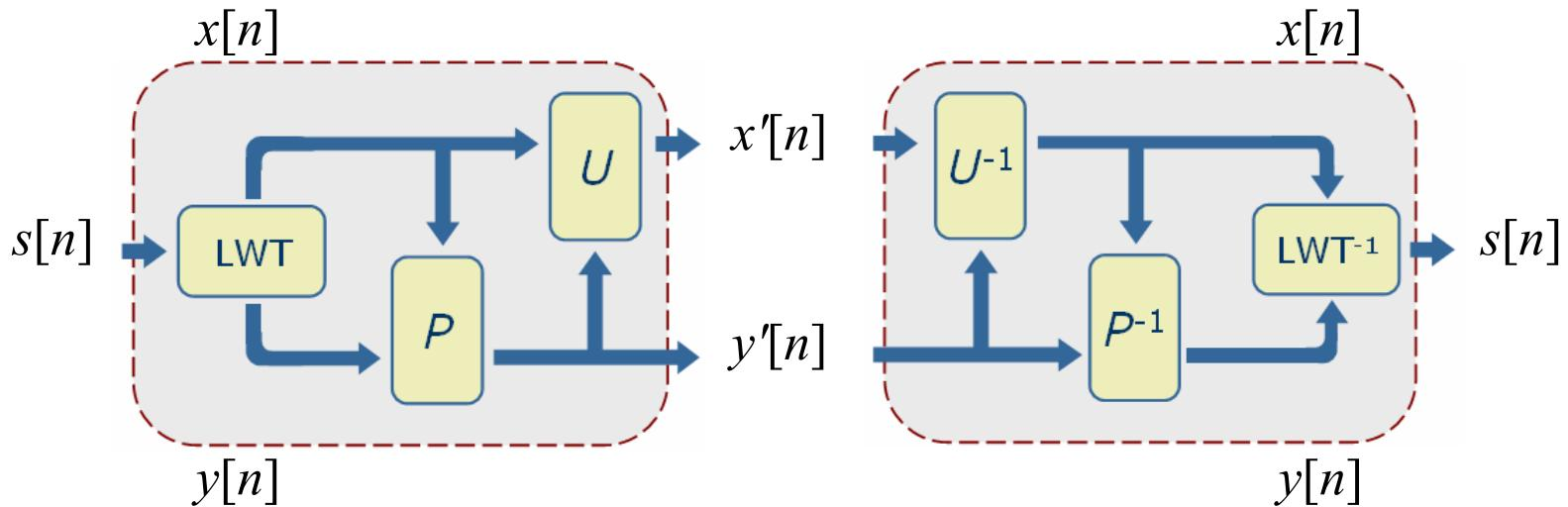
Detail signal:  $y'[n] = P(y[n], x[n - i])|_{i \in C}$
