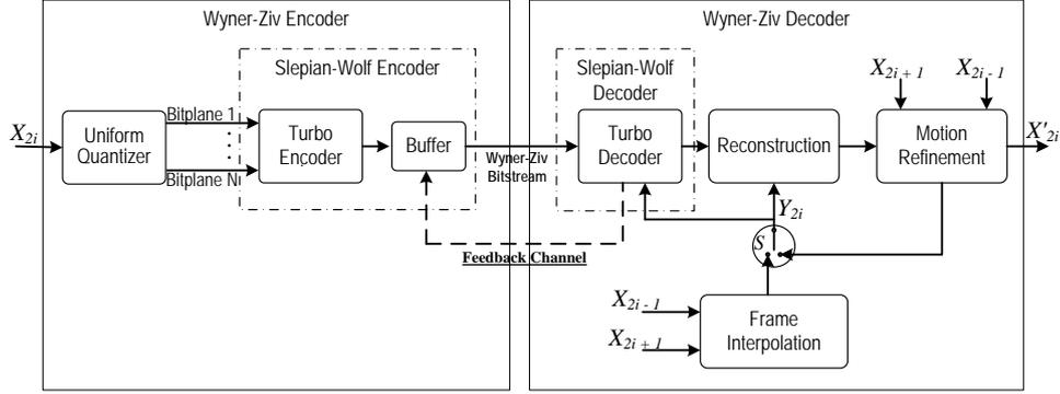
Figure 1: Block diagram of the IST-PDWZ codec
