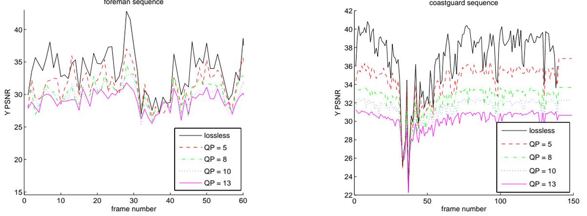
Figure 2: Quality of the motion-compensated interpolation: lossless vs lossy. The frame index refers to the interpolated frames only (odd frames). Left: *Foreman* sequence. QCIF@30fps (only the first 60 odd frames of *Foreman* are shown to avoid cluttering the figure). Right *Coastguard* sequence. QCIF@30fps
