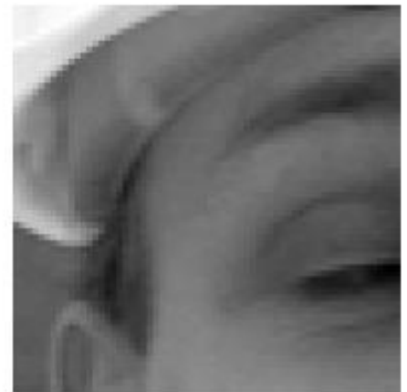
(f) Reconstruction with the 4,000 largest absolute values of the DCT coefficients.
