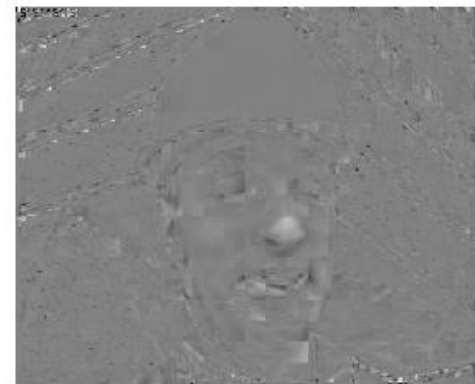
(c) Frame difference between the original and the intra predicted frame.
