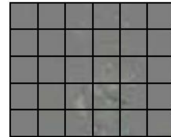
Difference between motion- compensated prediction and current frame u[x,y,t]
