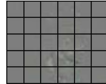
Difference between motion-compensated prediction and current frame u[x,y,t]
