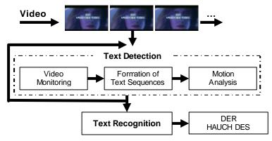
Fig. 1. Architecture of the proposed system.
