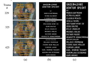
Fig. 3. Text extraction result for a video sequence: (a) video sequence; (b) text detection for individual frames (c) image resulting from the integration of the text in the full video sequence.
