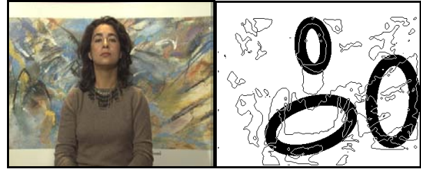
Figure 12 – False negative and false positives: original, contour colour segmentation and shape-based facial detection
